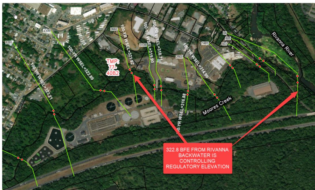
Figure 4: County Preliminary Model Cross Sections & 100-YR WSEL
